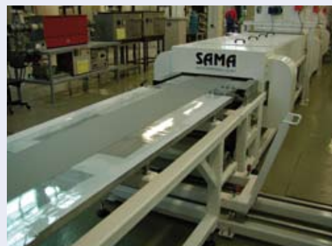
exit of the drying channel
