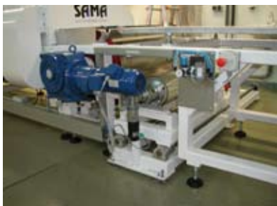
separation from ceramic tape and re-winding of the carrier tape
